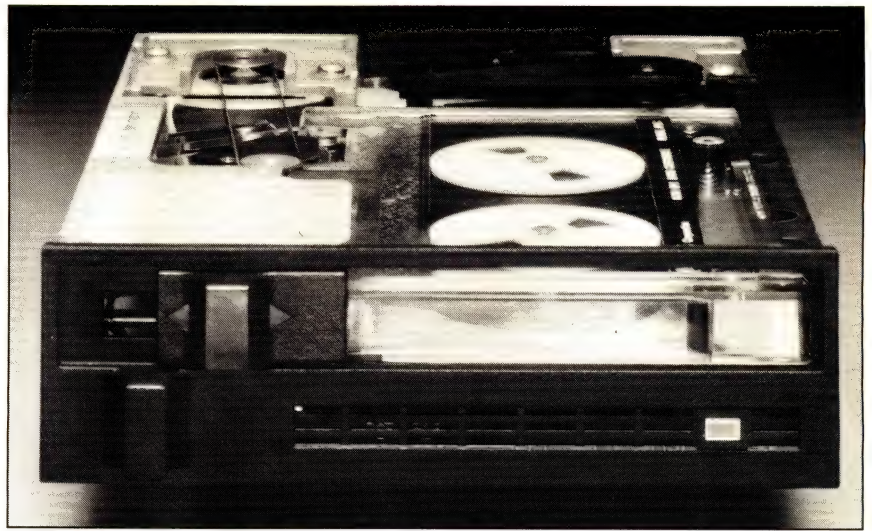
BACKUP. Archive's Scorpion 1/4-in. tape drive comes in 20-, 45-, and 60-megabyte capacities.
